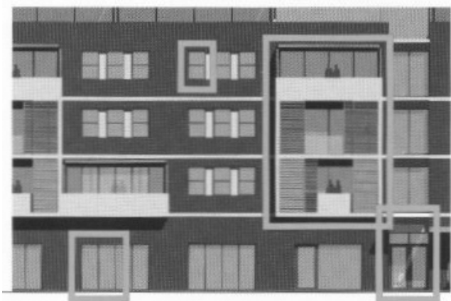
Figure B4. 6 Façade with vertical elements emphasised, window and balcony openings punched in masonry wall, and wall areas dominant
